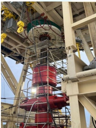
Illustration 2 Katch Kan Ecological Circular Tray Installed in Ixachi 89
